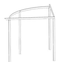
Slot the Rafter 1 and 7 onto the ends of the arc rafters as shown. Make sure that they in line with each other and the un notched post.
