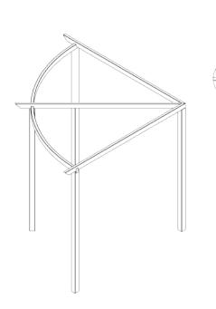
Place Rafter 4 so that the notch overlaps the join between the two arc rafters and sits on the un notched post central, between the other rafters.
